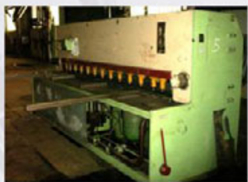
Name: SAN MACHINE Type: MG 31/16-20 Manufacturer: Maximum width: 3100mm Max material tick Dmax= 12mm Year of production 1981 Pieces: 1
