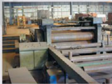
Name: Equipment for predeformation Type: Raddrizatrice 2000x30 Manufacturer: Di Parmigliari-Italy Max width 2000 mm Max thickness 30 mm Year of production 1981 Pieces: 1
