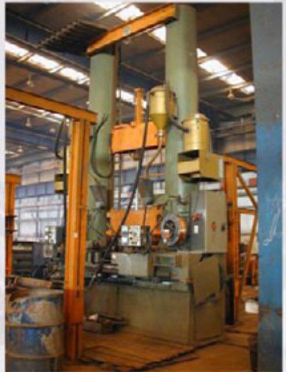
Name: Arc welding machine MASTER Type: ARMCO Manufacturer: ARMGO-Genova Italy Accessories: Aggregates (pcs=2) "IDEAL ARC" DC-1500 A, "The Lincoln Electric Company" -Cleveland, Ohio- USA, Steel profile dimensions: 700/200/3000 Year of production 1981 Pieces: 6
