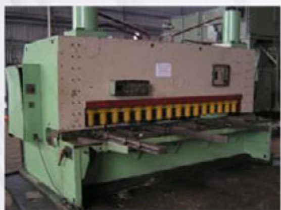
Name: SAN MACHINE Type: MG 31/16-20 Manufacturer: JELSINGRAD Max width B = 3100 mm Max material tick Dmax= 20mm Year of production 1981 Pieces: 1
