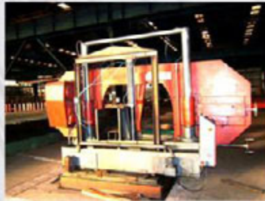
Name: ELECTRIC SAW Type: UMSY 1010 Manufacturer: Tyrkey Cutting capacity: 15-105m/min Year of production 2002 Pieces 1
