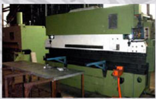
Name: BENDING MACHINE Type: Tip P1175 Manufacturer: TELEMQUANIQE Max length 4050 mm Max thickness 18mm Year of production 1996 Pieces: 1
