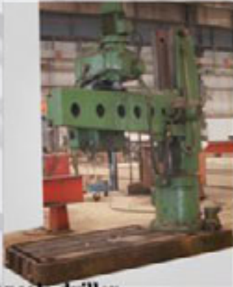
Name: Radial console driller Type: TRB 5A Manufacturer: TIGAR-SARTAH SCIG Max diameter of holes F max=50 mm 1 holes/min Year of production 1981 Pieces 3
